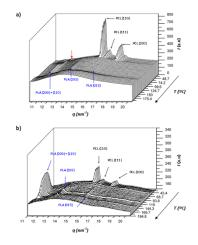
The disappearance of the Bragg reflections of the polycaprolactone crystalline phase and the subsequent cold crystallization process that rendered new Bragg reflections associated with the polylactide phase.
