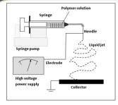
Electrospinning uses electrostatic forces (10-100 kV) to stretch a polymer dilute solution as it solidifies.
