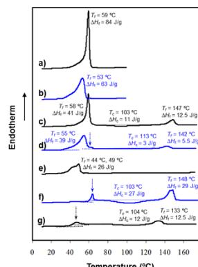
DSC heating traces of PCL/PLA-100 (a, b), PCL/PLA-50 (c-e) and triclosan unloaded (a, c, f) and 3 wt-% triclosan loaded (b, d, e, g) PCL/PLA-0 (f, g) samples. The second heating run of a triclosan loaded PCL/PLA-50 sample is shown in (e). Dotted arrows point out PLA enthalpic relaxation peaks.
