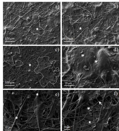
The three-dimensional porous structure of the microfiber mats supported cell adhesion and growth and how it was used by the cells to rapidly colonize the material. It is worth pointing out that cells can be clearly seen inside the material.
