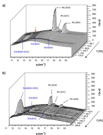
The disappearance of the Bragg reflections of the polycaprolactone crystalline phase and the subsequent cold crystallization process that rendered new Bragg reflections associated with the polylactide phase.
