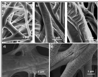
Scanning electron micrographs of electrospun samples revealed that unloaded samples with a high polycaprolactone content had a smooth surface, whereas small cracks were visible when the polylactide ratio increased, probably as a consequence of their higher stiffness. These cracks were predominant in the fiber bends. Triclosan loaded samples were characterized by a rough surface especially samples with a higher PLA content.
